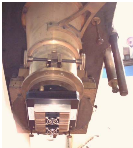
Fig. 2 - Apogee AP47P CCD Camera mounted on the optical telescope
